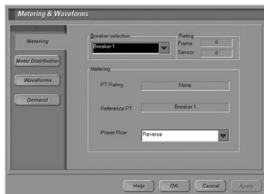
Figure 8.8 Configuration Information for Metering
